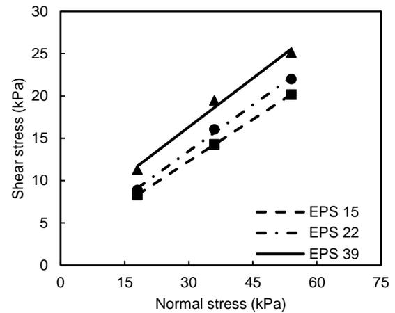
Figure 9. Mohr-Coulomb failure envelopes of geofoam-PVC interface
