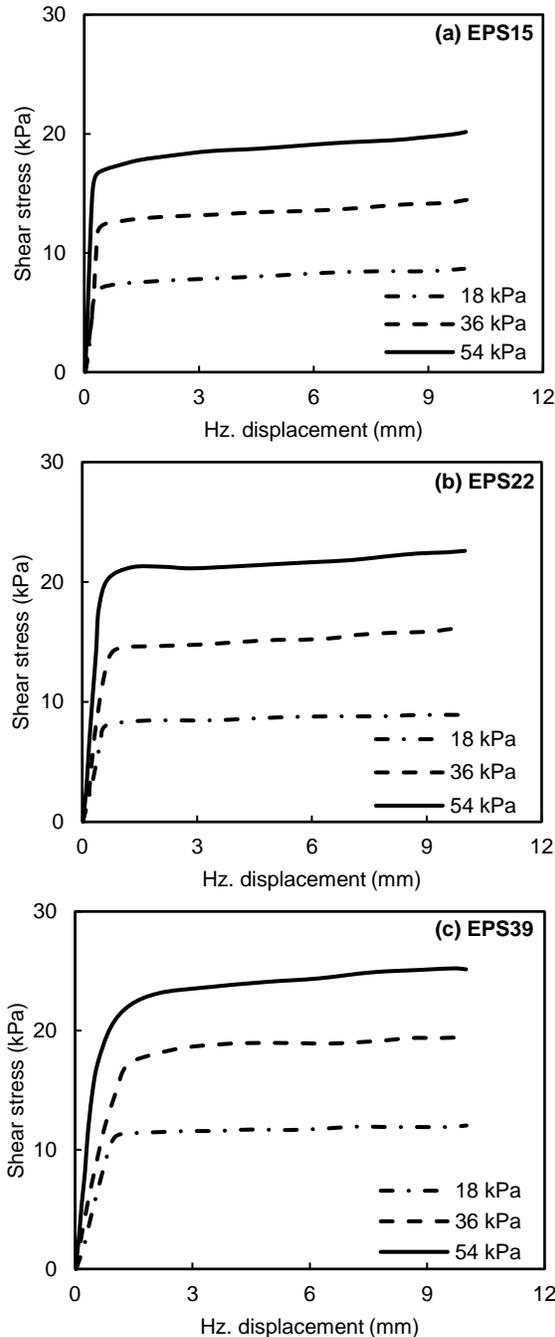
Figure 8. Shear stress vs Hz. displacement for geofoam-PVC interface with densities that range from 15 to 39 kg/m<sup>3</sup>
