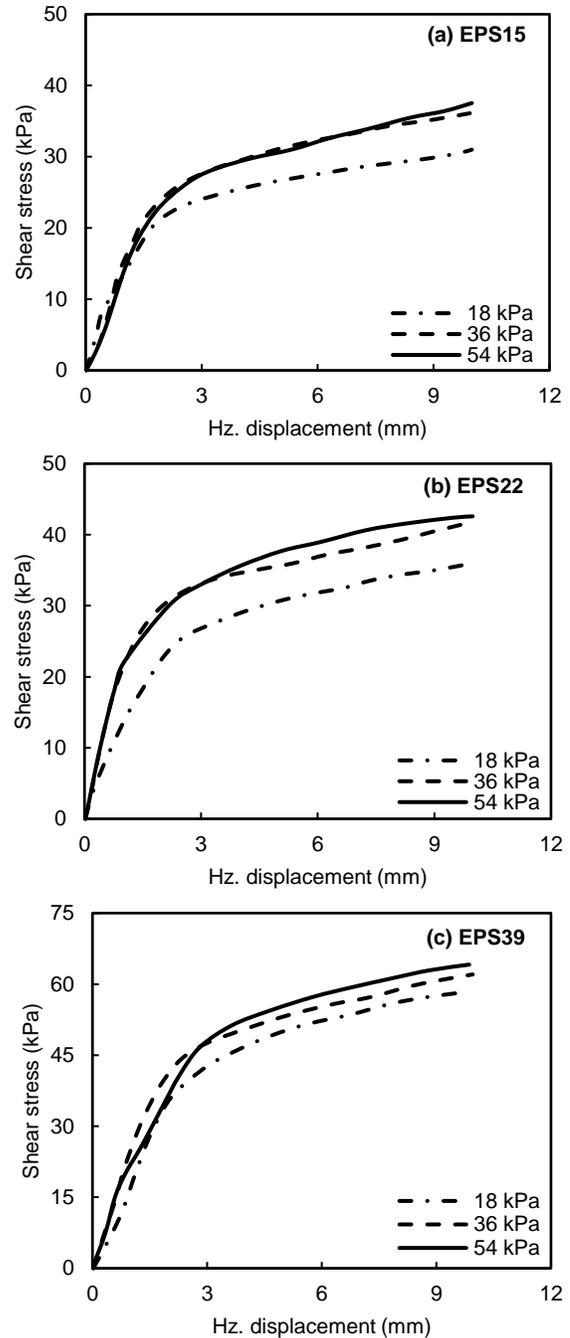
Figure 3. Shear stress vs Hz. displacement relationships for monoblock geofoam having densities that range from 15 to 39 kg/m<sup>3</sup>
