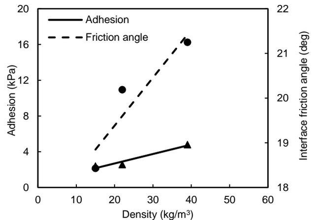
Figure 10. Adhesion and interface friction angle as function of the geofoam density for geofoam-PVC interface
