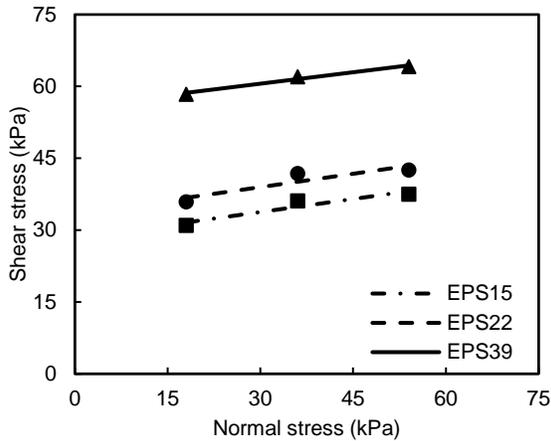
Figure 4. Mohr-Coulomb failure envelopes of monoblock geofoam sample
