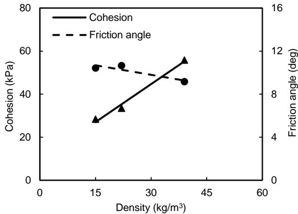
Figure 5. Monoblock cohesion and friction angle as a function of the geofoam density
