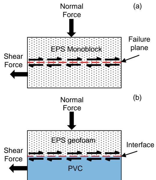
Figure 2: Schematic diagram of (a) Monoblock direct shear test; (b) Interface direct shear test
