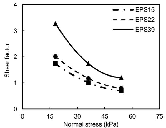
Figure 7. Shear factors for EPS15; EPS22 and EPS39 monoblocks
