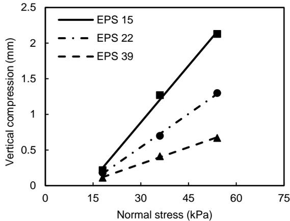
Fig 11. Vertical compression vs Normal stress for geofoam-PVC interface
