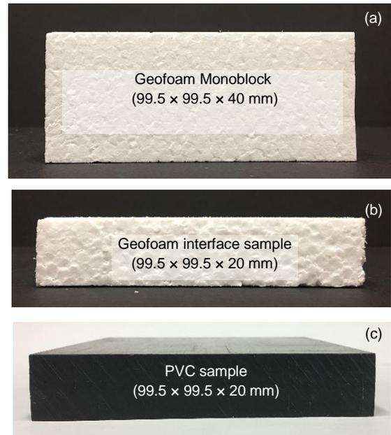
Figure 1: (a) Geofoam monoblock; (b) & (c) geofoam and PVC samples used in the interface tests
