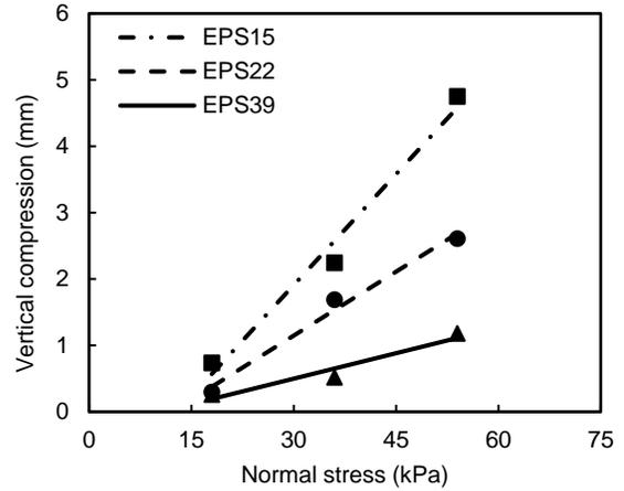
Figure 6. Vertical compression vs Normal stress for monoblock geofoam
